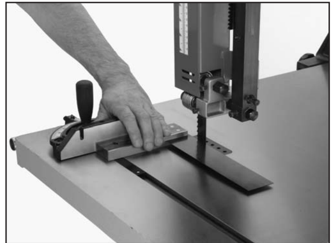
Figure 17. Squaring miter gauge to blade.
